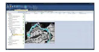
Part History provides pass/fail results, waveform or image characteristics and feature checks on a single serial number for reporting or additional investigation.
