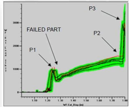
sigPOD screen showing Bushing Press PASS/ FAIL signatures
