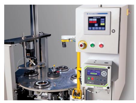
C20 integrated into an automated test cell
