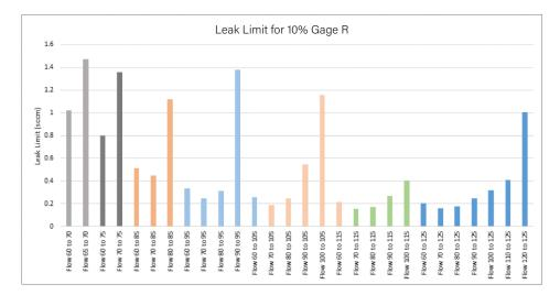
This graph, produced using Sciemetric's QualityWorX data analysis tools, shows a comparison of leak rate vs. gage R with gage R constant at 10%. This data enabled the manufacturer to clearly see the impact of shortening cycle time and how it would affect the leak rate and the gage R.
