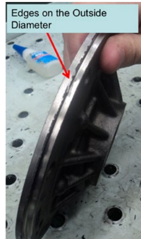
Figure 5 and 6 – Example defects caused by worn machine tooling
